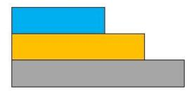
PET Release Liner (23µm) Adhesive Layer (10µm) Base PET Film (50µm)
