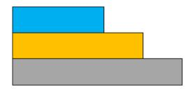
PET Release Liner (125μm) Adhesive Layer (15μm) Base PET Film (38μm)
